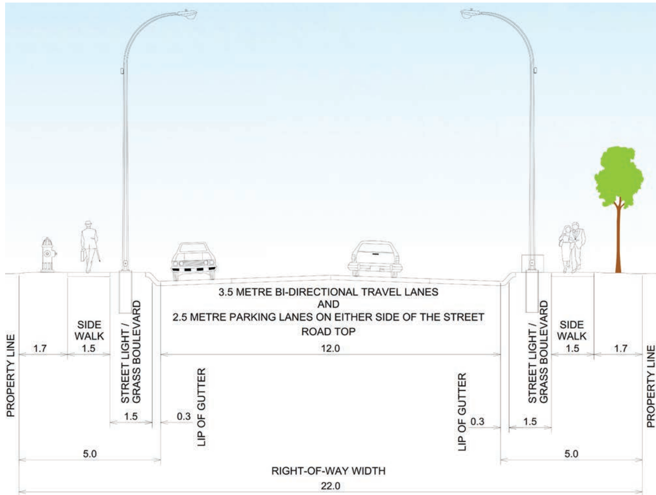
Figure 1: Collector Roadway Typical Cross Section
