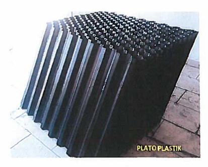
The manual cleaning process results in damage to the lamellas which are made of a polycarbonate material. The lamellas at the Water Treatment Plant have been damaged to the point that they require replacement.
