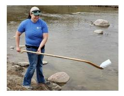
Dallas Peters, former SCCWS Watershed Technician collecting samples to test for levels of phosphorous in the water in the Swift Current Creek.
