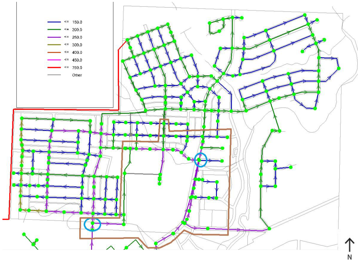
Figure 17 Proposed North East Water Supply Network (the existing network in the study area is shown under the brown polygon)
